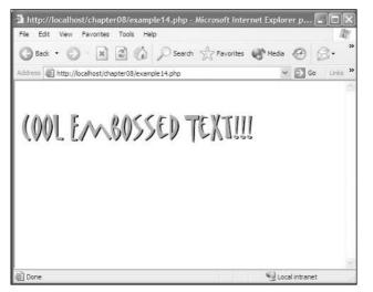
Figure 8.14 Creating cool text effects with the ImageTTFText() function.
