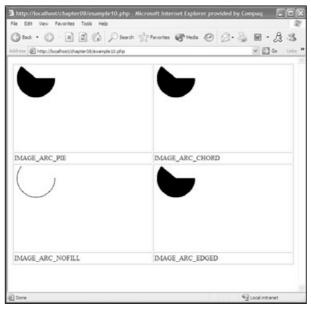
Figure 8.10 The ImageFilledArc() function.
