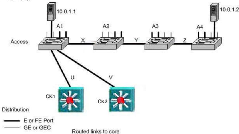
The diagram shows a wiring closet stack of four L2 switches A1, A2, A3, and A4. A1, A2, A3 and A4 are connected in series. Switch A1 is the root switch and connects to CK1 and CK2. There are no loops in the wiring closet VLAN (=subnet). The architect wants to remove X, Y and Z, and connect A1 directly to A2, A3, and A4 in a star. Is this a good idea?
