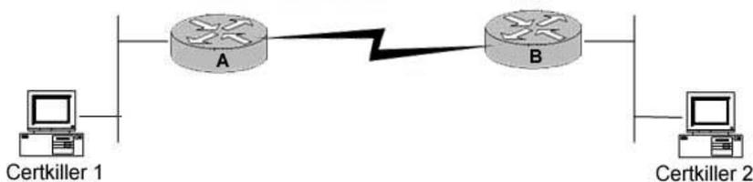
Certkiller 1 and Certkiller 2 are on Ethernet LANs in different buildings. A serial line is installed between two Cisco routers using HDLC serial line encapsulation. Routers A and B are configured to route IP traffic. Certkiller 1 sends a packet to Certkiller 2. What is the destination MAC address of the packet on Certkiller 1's Ethernet?
