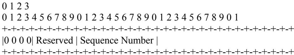
In the above diagram, the first 4 bits MUST be set to 0 to indicate PW data. The rest of the first 16 bits are reserved for future use. They MUST be set to 0 when transmitting, and MUST be ignored upon receipt.
