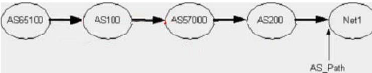
Using the above diagram, which are valid BGP AS\_Path Attributes received at Net1 for a route originating from AS65100? (multiple answer) Select three.
