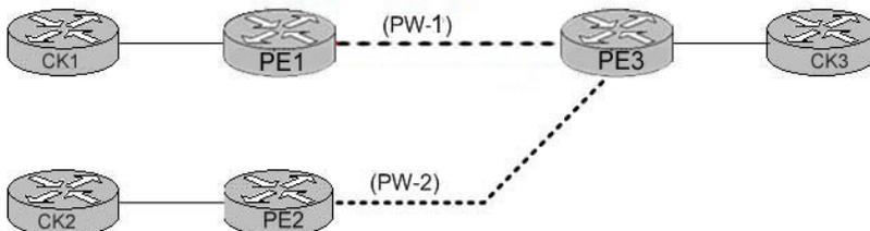
PE1 and PE2 provision point-to-point EoMPLS pseudowires PW-1 and PW-2 to PE3, and both pseudowires have VC ID 100. PE3 provisions a multipoint VFI with a VPN ID 100. Which statements are correct? Select two.
