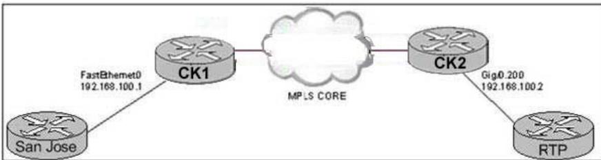
CK1 and CK2 are connected to the MPLS cloud. All MPLS tables from CK1 and CK2 are working. Observing the shown topology, will this scenario work?
