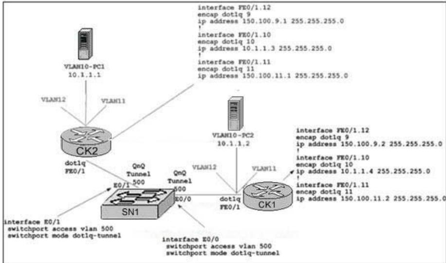
What is true about the SW1 configuration, with respect to communication between PC1 and PC2?
