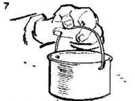
PUNCH HOLE WITH NAIL TO INSERT HANDLE OF FAIRLY HEAVY WIRE BEND HANDLE TO FIT
