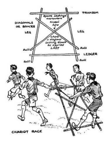
The design we have shown is perfectly adequate carried out in light timber, but if you are using heavier spars then it is worth bearing in mind that in the interests of balance it is quite a good plan to put the diagonal braces with the three points on the opposite side to the transom and the ledger.
