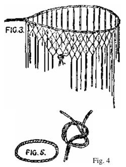
Care should be taken in the spacing to see that no clipped mesh comes directly under another of its kind. After fixing a rod to the desired length, the net is complete.
