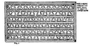
The type of lay-out described here can be used for both Sennit and Rush work, and should be made according to the use the mat is to be put to. Sennit is a flat plait made of coco-nut fibre and is suitable for rough outdoor wear. Its formation as a mat allows for the removal of dirt and stones quite easily.
