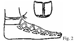
The back of the sandal, shown in Figure 2, has to be stitched with two needles. Buy from your shoemaker an awl, a length of waxed thread and two leather-work needles, which are a little stronger than ordinary ones and have blunt points. The awl is used for making holes in the leather
