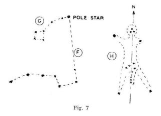
Also in the northern sky is Orion, supposed to be a man with a belt and sword (Fig. 7H). A line through the sword and the head points N. However, Orion is much farther from the Pole Star than The Plough, and is more difficult to use. Remember that the Pole Star stays still and all the other stars appear to revolve around it. Consequently, do not expect to necessarily see a constellation the same way up as I have drawn it.
