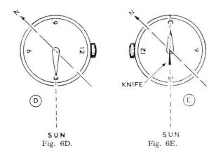
It appears to curve through the sky from E. through S. to W. and intermediate points can be estimated according to the time, *e.g.*, at 9 am. it is S.E. Remember to allow for summer time if that is in force, making noon at 1 p.m. and using 7 instead of 6 o'clock.
