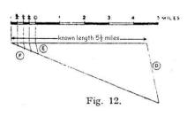
through the 1 mile mark (Fig. l2E). Use a pair of dividers to step off the number of miles you want on the scale.
