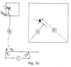
The two methods can be combined. Triangulation should give complete accuracy, but the grid will serve as a general guide. It also provides a check on any slip in setting the compasses. It is possible that a few points will come exactly on grid lines, so they may be fixed without work with the compasses.
