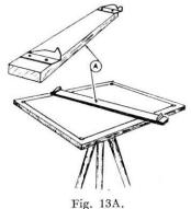
straight edge fitted with sights. The longer the rule and the farther the sights are apart, within reason, the more accurate can you work. The sights may be made from pieces of tin tacked on. The important thing is that they should come over the drawing edge (Fig. 13A). No other tools are essential, but another rule for measuring and a compass for checking and setting the board may be useful. The paper should be fixed down with pins and drawing done with a sharp hard (2H) pencil.
