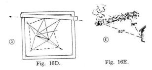
Using compass triangulation, the fixing of points out of sight of the first stations is simple. Move to a point already fixed, but within view of the chosen point and take a bearing of it. Transfer this with the protractor. If a second bearing is needed, move to another known point and do the same again (Fig. 16E).
