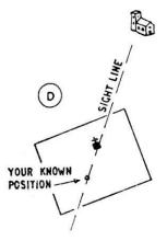
If you can see several landmarks which you can identify on the map, you can set it without using a compass. If you can only see one landmark and you know where you are on the ground and on the map, you can set the map. Several landmarks help to check each other, or you can use an odd landmark to check your setting by the compass.
