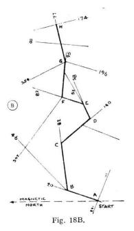
along that cross bearings of prominent landmarks may be possible from points widely different on the route and in separate sections. There is less risk of error in cross bearings that are somewhere near right-angles to each other than in those which are very acute or obtuse. Within reason, the more bearings you can take of an object, the better, as they serve to check each other. However, expect a slight error—it is unlikely that all bearings will cross at an exact point.
