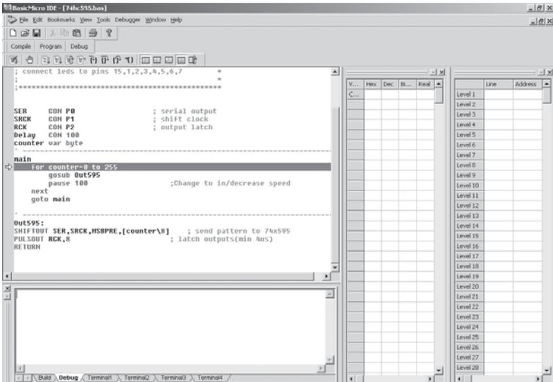
Once you have entered the program, save it. Make sure the target device is connected and power is applied. Next, click the “Debug” button on the tool bar.
