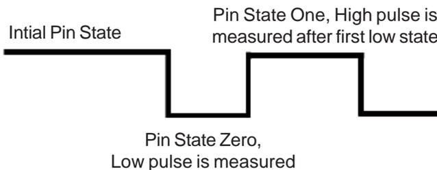
PULSIN will return the pulse width in  $\mu\text{s}$ .
