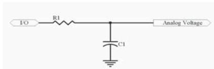
The capacitor will hold the voltage set by PWM after the instruction has completed. How long it holds the voltage will depend on how much current is drawn, by external circuitry, and internal leakage of the capacitor. In order to hold the voltage the program must periodically repeat the PWM instruction to give the capacitor a refresh charge. The PWM command lets you set the charging time in terms of PWM cycles.
