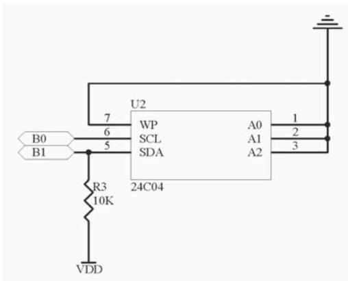
This next I2c EEPROM program demonstrates the I2Cin and I2cout commands. This program will record the state of pin A0 over a period of time and play it back on pin A1. It was designed for use with the 512 byte EEPROM 24C04
