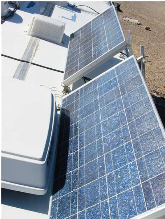
Minus 6.4 amps from these two panels!! This is 90 % of the output of a full panel.
